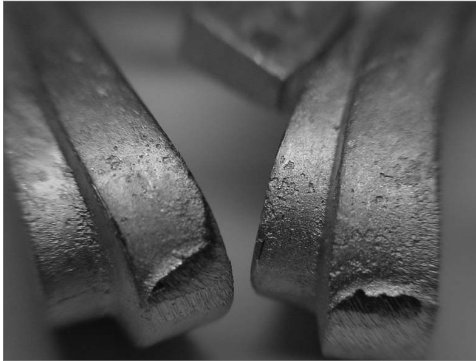
Figure 17 Investment defect from steam dewaxing with water level too high
