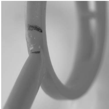
Figure 3 Wax pattern with mold defect caused by solder pit in master model
