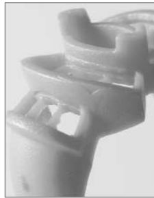
Figure 6 Rough surface on wax pattern from dirty mold
