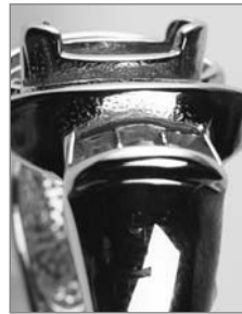
Figure 7 Casting from defective wax pattern still shows rough surface
